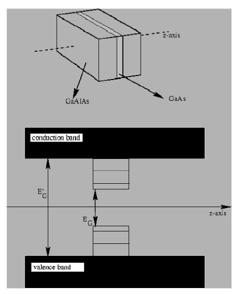
Figure 4.4: A schematic representation of a quantum well
